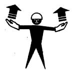
to raise pile, hammer, and leads together, use both hands palms upward in upward motion.
