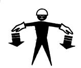
to lower pile, hammer and leads together, use both hands palms downward in down motion —
